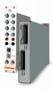
The new **satellite module** has 4 inputs allowing the reception of 4 different satellite bands per module. Because the module has 8 satellite tuners and a built-in multiswitch, reception of 8 different transponders coming from any of the 4 input satellite bands is possible.
