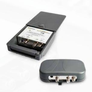
The **Stacker-Destacker** is the perfect solution to upgrade an old single-cable system with a twin (or quad) LNB to be used in combination with a dual input receiver (PVR) or 2 separate single input receivers. The advantage of using the Stacker-Destacker is that you don't need an additional cable. The Stacker converts the frequencies of the second input, so it is literally stacked above the frequencies of the first input. The Destacker converts the frequencies back to the original ones.
